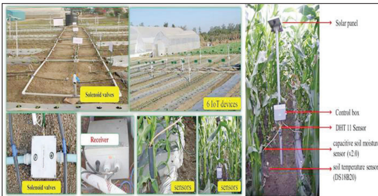
Fig. 2 IoT based irrigation system
