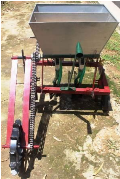
Fig. 3: Developed animal drawn seed drill
