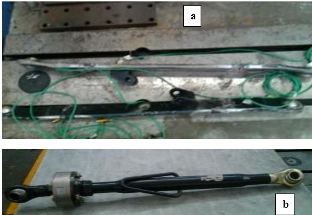
Fig. 1. Instrumentation for measurement of force (a) Strain gauge on lower links (b) Load cell on top link
