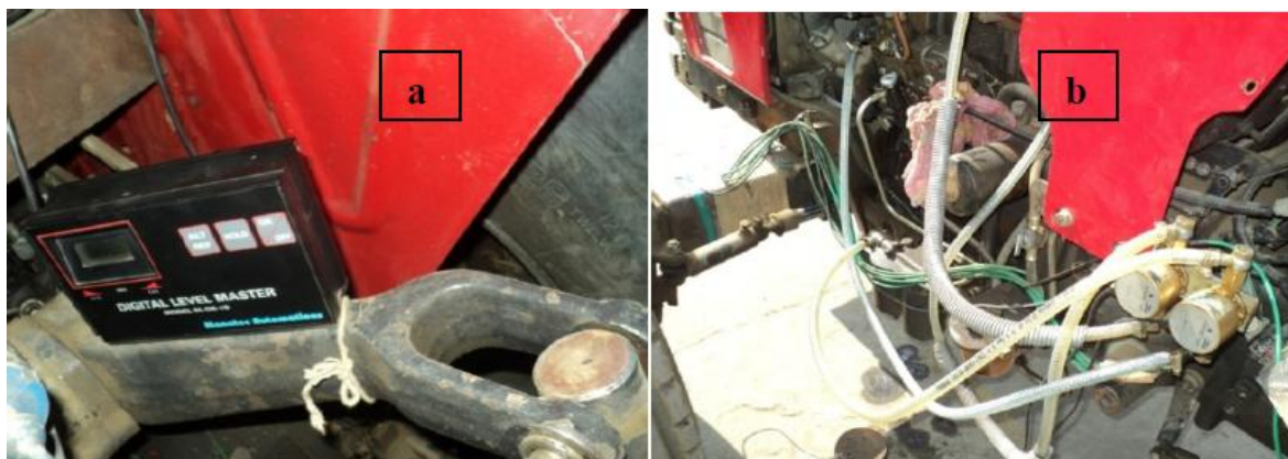
Fig. 3. Instrumentation for working depth and fuel consumption measurement (a) Digital level meter and potentiometer mounted on rocker shaft, (b) Fuel flow meter installed on the tractor
