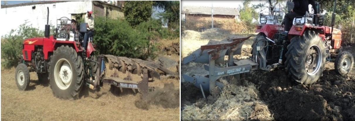
Fig. 5. Field operation with 3-bottom and 2-bottom reversible plough
