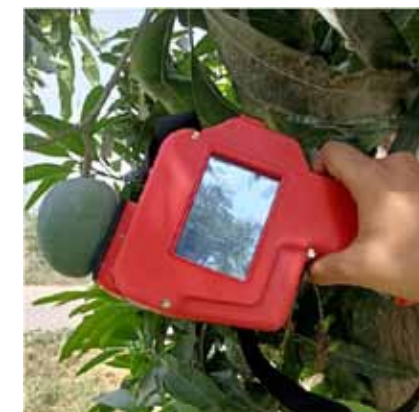
Fig. 2. Indigenous hand held mango maturity and ripeness level tester
