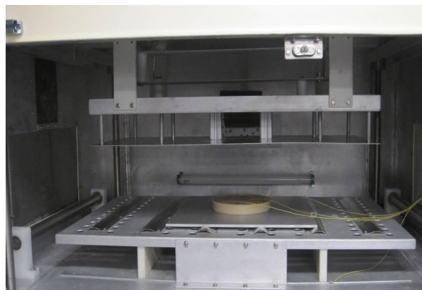
Fig. 1: Pilot-scale 6 kW, 27.12 MHz RF unit showing the two-pair plate electrodes
