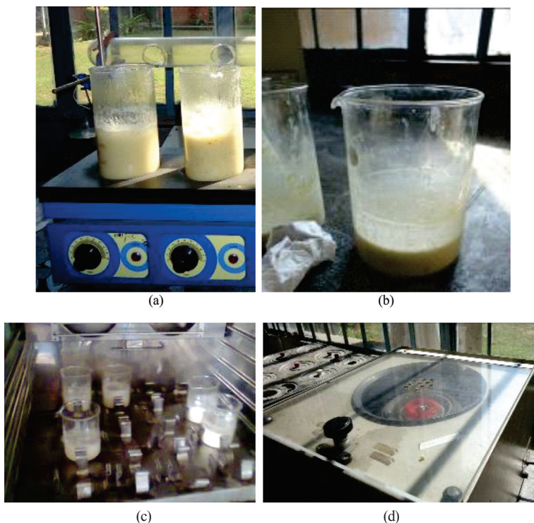
Fig. 3: EAAE maize germ oil extraction (a) cooking of ground germ in distilled water, (b) cooling of cooked slurry, (c) hydrolysis of enzyme buffer solution with cooked slurry, and (d) centrifugation of processed slurry
