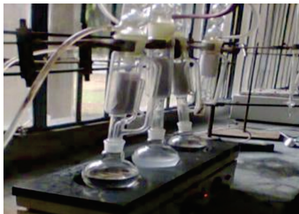
Fig. 2: Maize germ oil extraction using solvent extraction process
