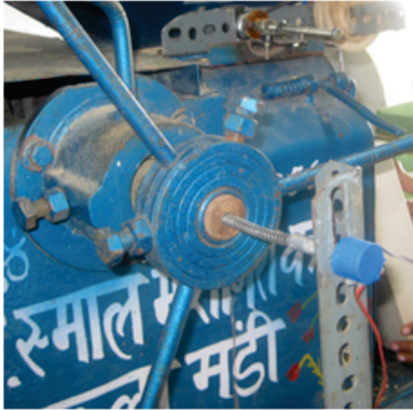
Fig. 1: Potentiometer as a sensor to read roll clearance
