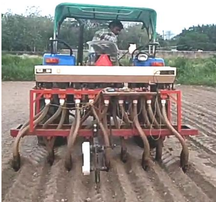
Fig. 8: Field evaluation of planter with sensor system
